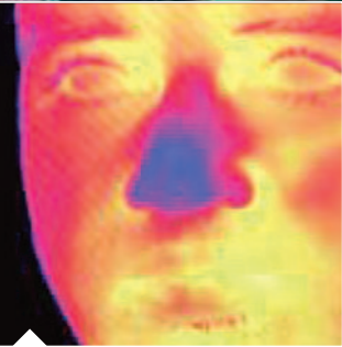
INSET IMAGE: The ISMS thermal camera monitors facial temperature modulation of the crew while performing typical pilot tasks.
